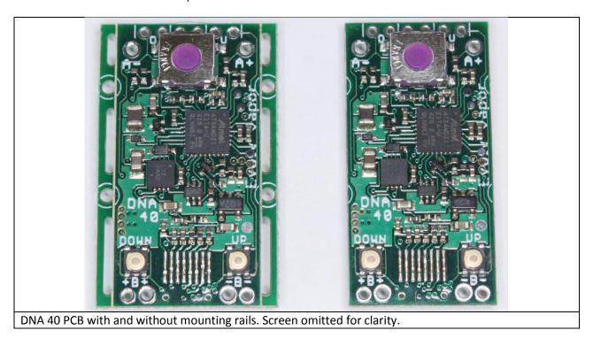
The mounting rails have .063" diameter holes drilled for mounting screws. #0 or M1.6 screws are recommended.
