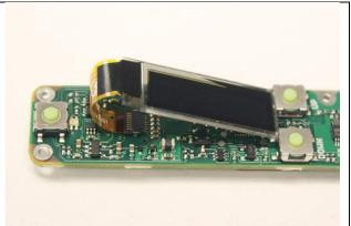
**Step 4:** Close the locking tab and press until the connector gently clicks. Remove the clear screen protector by pulling on the colored tab.
